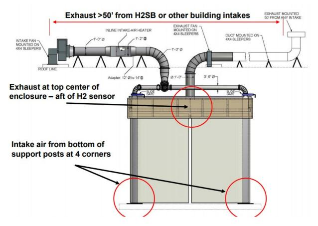
The graphic above illustrates the ventilation strategy for the service bay. During normal operation, air exchange is continuous; an intake takes outside air and introduces it near the floor of the enclosed area. In the event of a hydrogen alarm, the rate of air exchange is increased dramatically in order to dilute and extract any hydrogen through the exhaust of the enclosure. The exhaust vent is located at least 50 feet away from the ventilation system intake.
