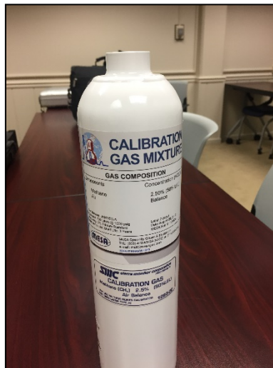
Figure 13: Calibration gas for detector calibration.
