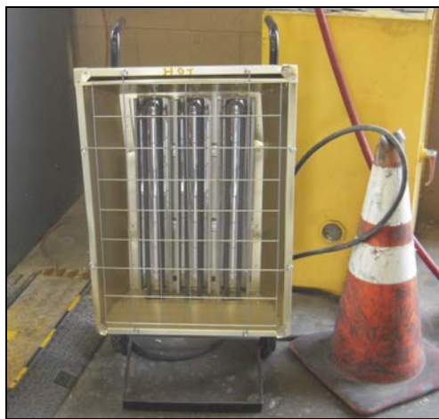
Figure 10: Floor-mounted portable propane heater. Photo courtesy of Gladstein, Neandross & Associates, NREL
