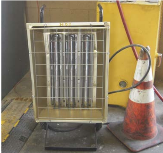
Figure 21: Floor-mounted portable propane heater. Note the exposed heating elements. Photo courtesy of Gladstein, Neandross & Associates, NREL
