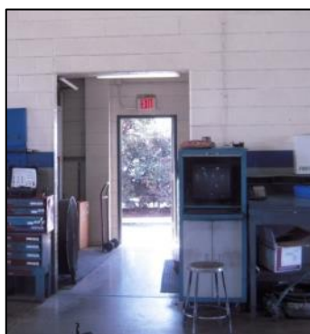
Figure 33: A potential path of migration created by an open passageway. Photo courtesy of Gladstein, Neandross & Associates, NREL
